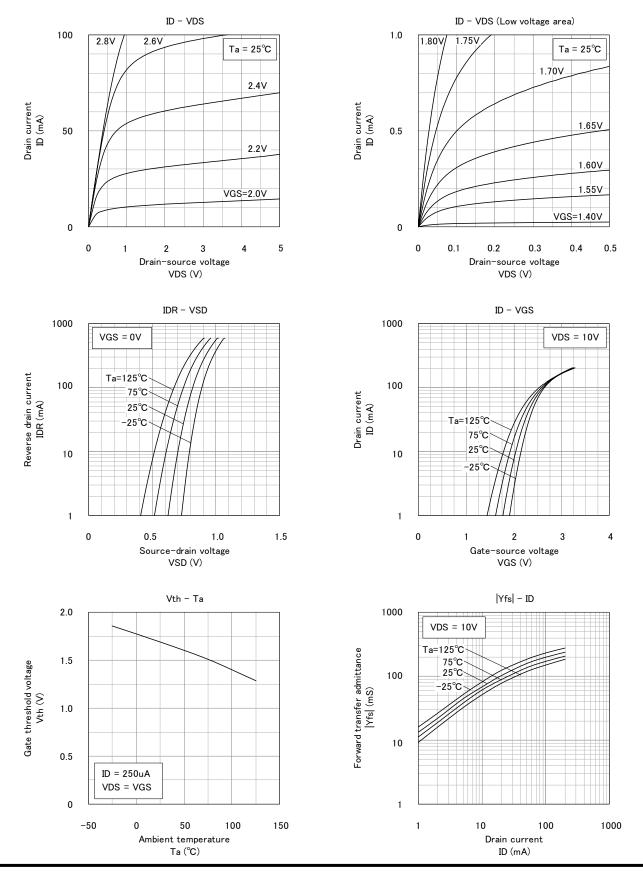
High Speed Switching Silicon N-channel MOSFET
