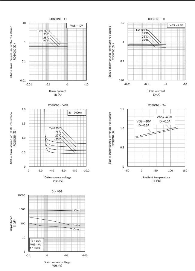
High Speed Switching Silicon P-channel MOSFET
