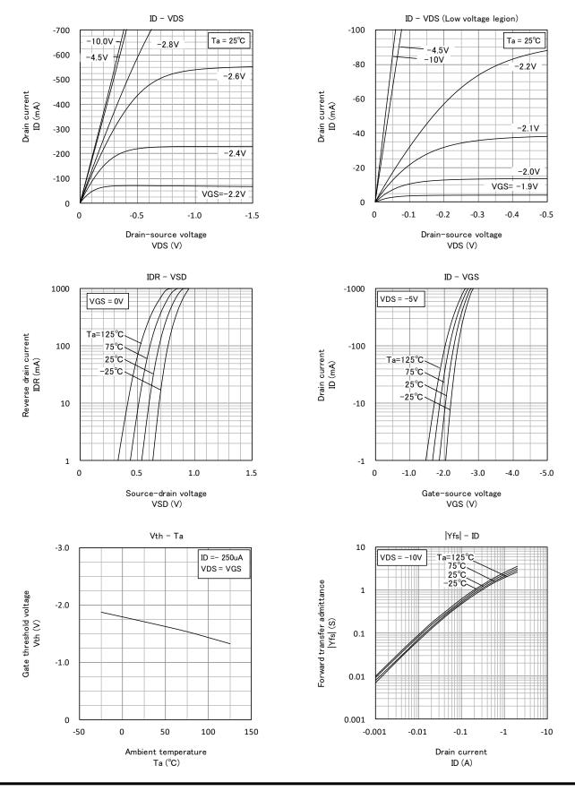
High Speed Switching Silicon P-channel MOSFET
