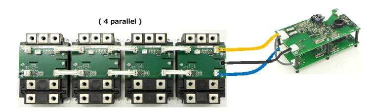
Note) The harness for connections doesn't attach at the time of shipment.
