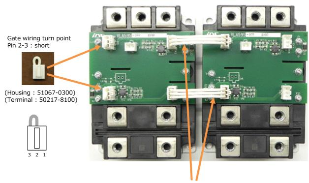
Unit connection harness (Housing: 51067-0300) (Terminal: 50217-8100)
