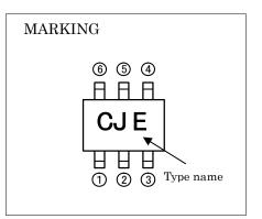
Dual Transistor For Differential Amplify Application Silicon NPN Epitaxial Type
