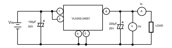
Please use electrolytic capacitor of output side with high frequency and low impedance.
