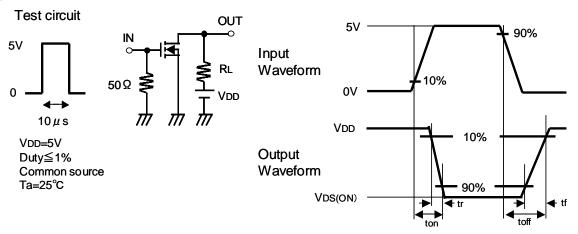
High speed switching Silicon N-channel MOSFET
