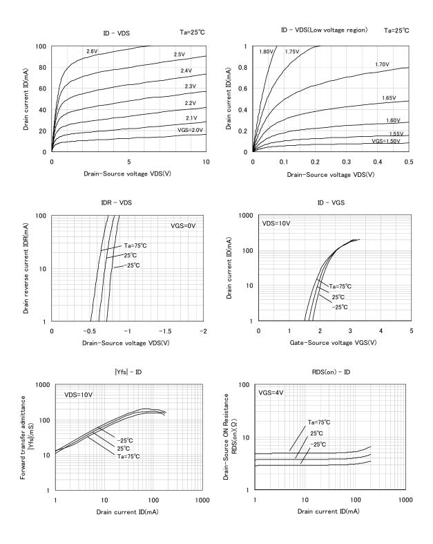
High speed switching Silicon N-channel MOSFET
