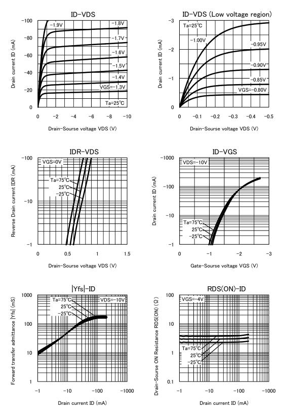
High speed switching Silicon P-channel MOSFET
