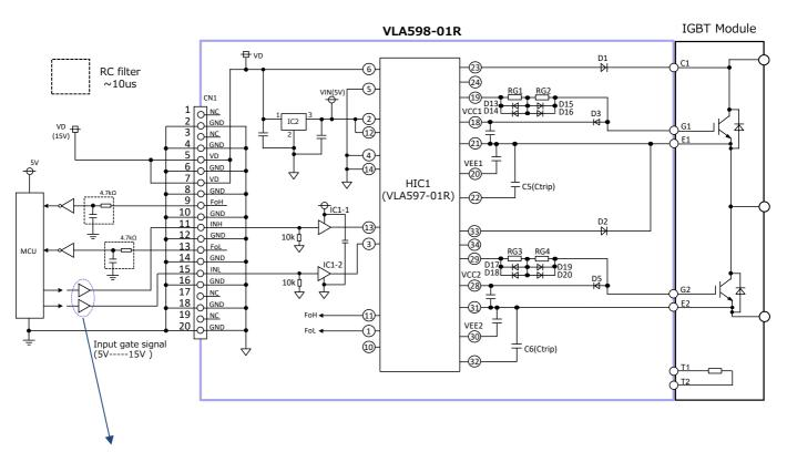
Note) About the IC which drives gate signal on input side, it is not recommended to use the one whose output is open collector or open drain type.
