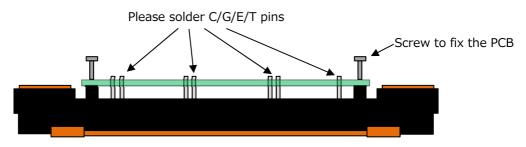
Note) Temperature of soldering iron tip: 360°C (max) under 5 seconds
