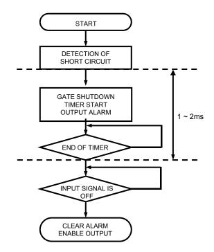
(1)In case the gate voltage is "H" and the collector voltage is high, the gate driver will recognize the circuit as short circuit and immediately reduce the gate voltage.(Slow shut down) Besides, put out an alarm sign which inform that protection circuit is operating.
